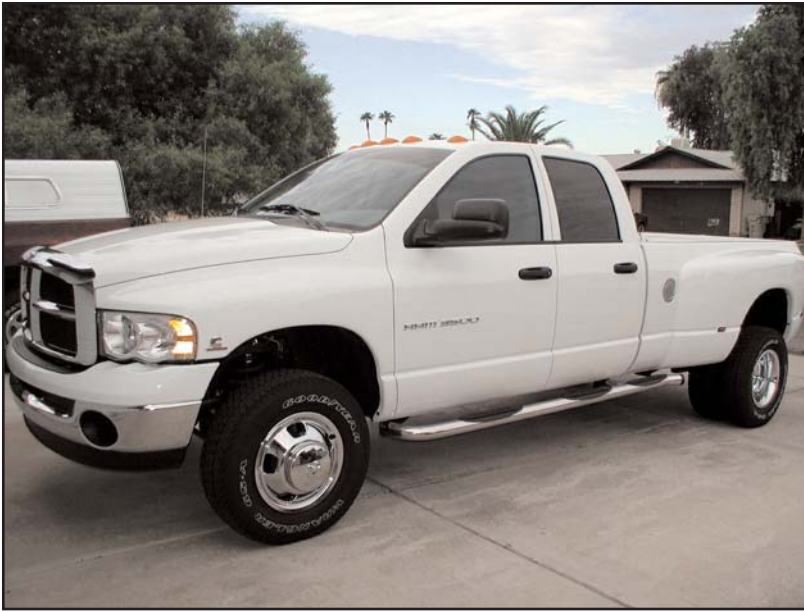
Improved nerf bar design from Willmore Manufacturing incorporates a step pad without compromising the strength or integrity of the steel tube.
