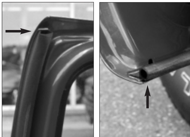
The Dodge Durango utilizes seals that are attached solely with 3M™ Weatherstrip Attachment Tape on both the B-Pillars and lower door dust seals on all four doors.
