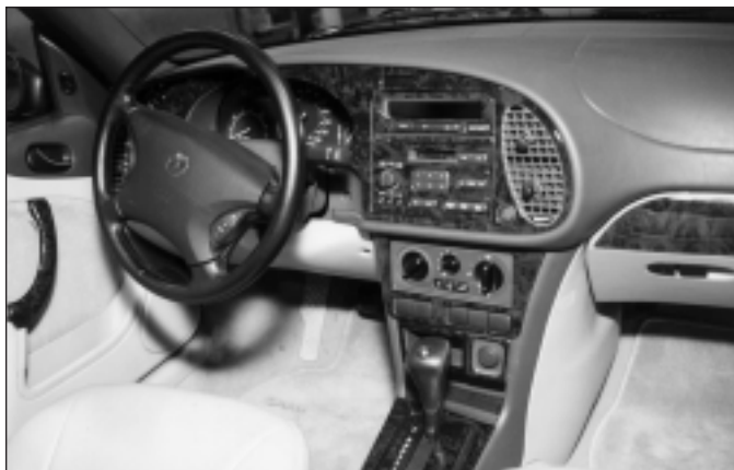
This 1999 Saab 93 convertible features a burled walnut dash kit from Spectrum Accessory Distributors, installed using 3M™ Primerless Acrylic Foam Tape 5568 for permanent attachment without the use of adhesion promoter.
