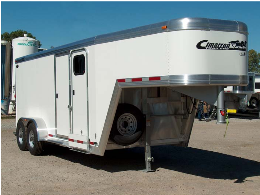
Cimarron Trailers’ Transtar model also uses 3M™VHB™ Tape to achieve the smooth-sided appearance
