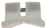
The unique debonding slot concentrates stress at the base of the bracket, causing it to collapse under gentle pressure.
